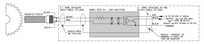
Note: Both magnetic pickup leads must be floating.
